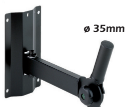
EU-03433 Adjustable wall support for SPEAKON version only - Arm : W320 x H120 x ø 35 mm - Wall plate : W140 x H250 mm - Rotation : 0 - 120° / Tilt : 0 - 45°
